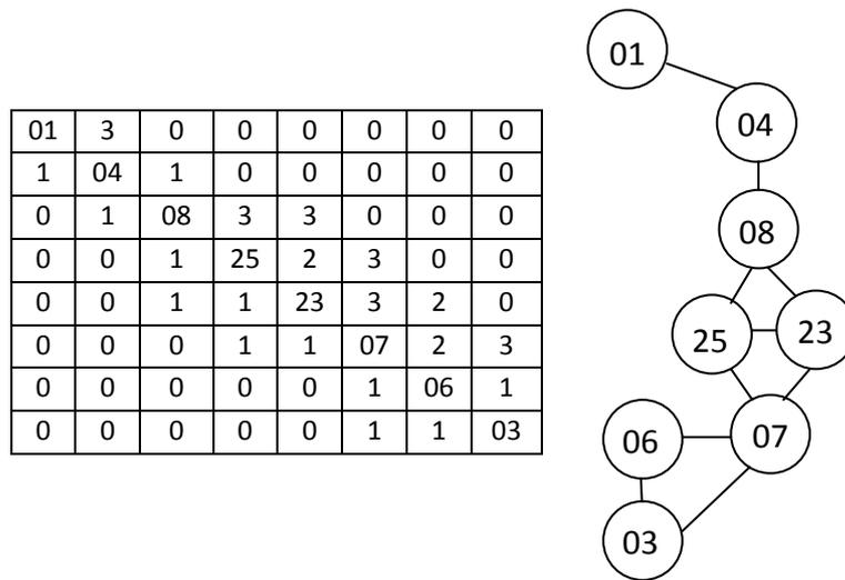
**Fig. 6. Feasible final structure of packing machine obtained with GA**
