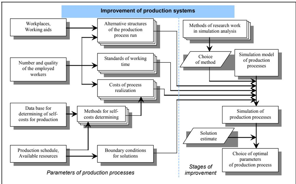
Fig.2. Input data bases for calculations and determination of optimal parameters in simulation analysis
