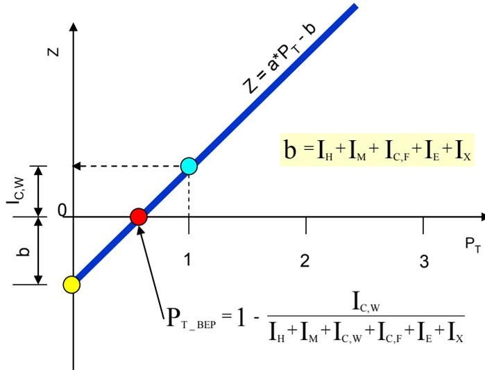
Fig.2 Analysis Model of  $P_{T\_BEP}$
