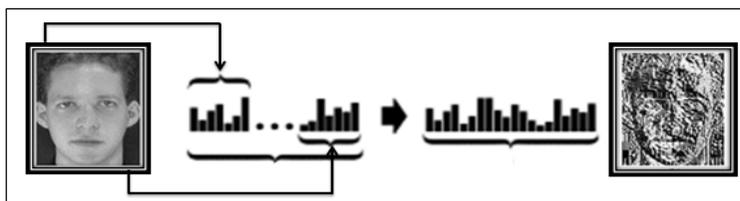
**Fig. 3. Extracting feature histogram from the face image**
