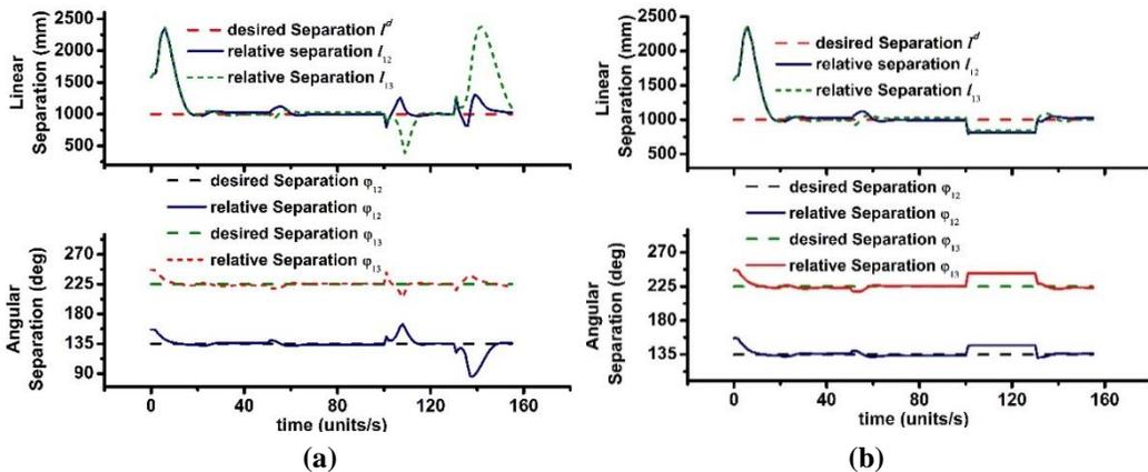
Fig. 6. (a) Linear and angular separation of robots in wedge-shaped formation exhibiting loss of formation using generalized tracking controller; (b) Linear and angular separation of robots in wedge-shaped formation exhibiting tightly coupled separation using proposed controller during backward motion
