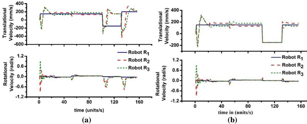
**Fig. 7. (a) Velocity profiles of robots in collateral formation exhibiting uncontrolled velocities using a tracking controller; (b) Velocity profiles of robots in collateral formation exhibiting controlled velocities between the robots using the proposed controller during backward motion**
