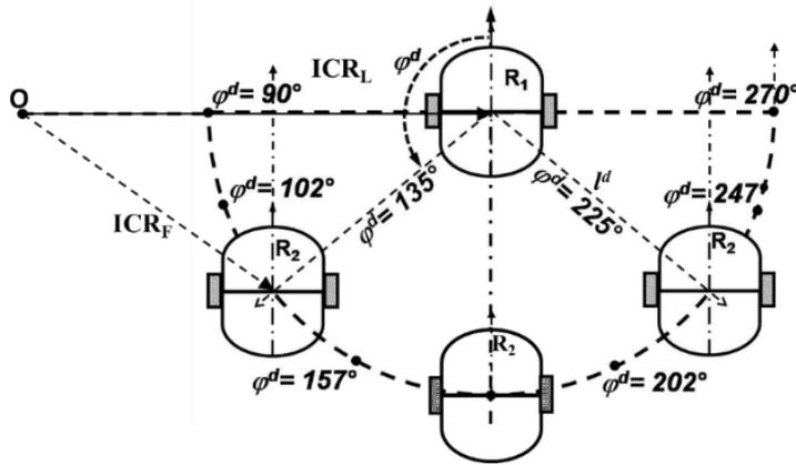
**Fig. 2. Position of Robots in desired linear and angular separation describing the formation topologies**
