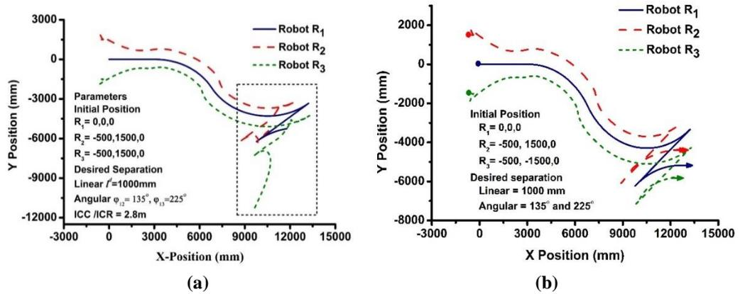
Fig. 5. (a) Trajectory of robots in wedge-shaped formation exhibiting uncontrolled motion using a tracking controller; (b) The trajectory of robots in wedge-shaped formation exhibiting controlled motion using proposed controller during backward motion
