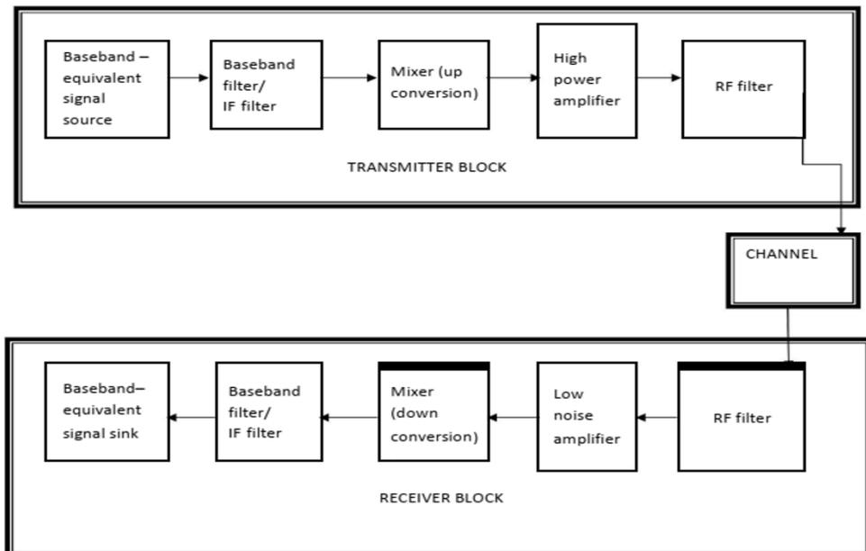
Fig. 1. Novel design of the low-IF-front Wi-Max transceiver
