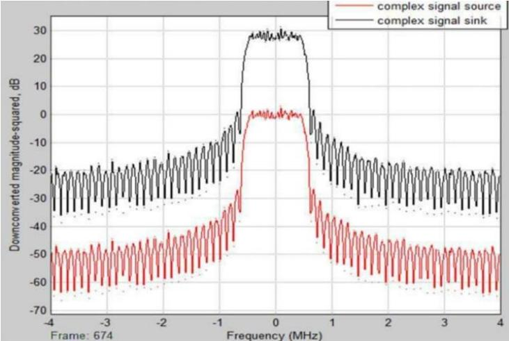
**Fig. 4. Modulated QPSK signals transmitted and received**
