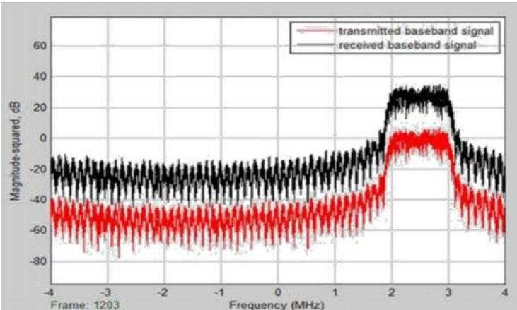
**Fig. 5. Transmitted and received spectrum of base-band signals**
