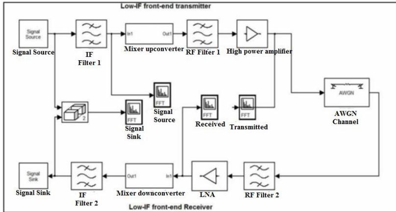
Fig. 2. Simulated model Low-IF-RF front end Wi-Max transceiver
