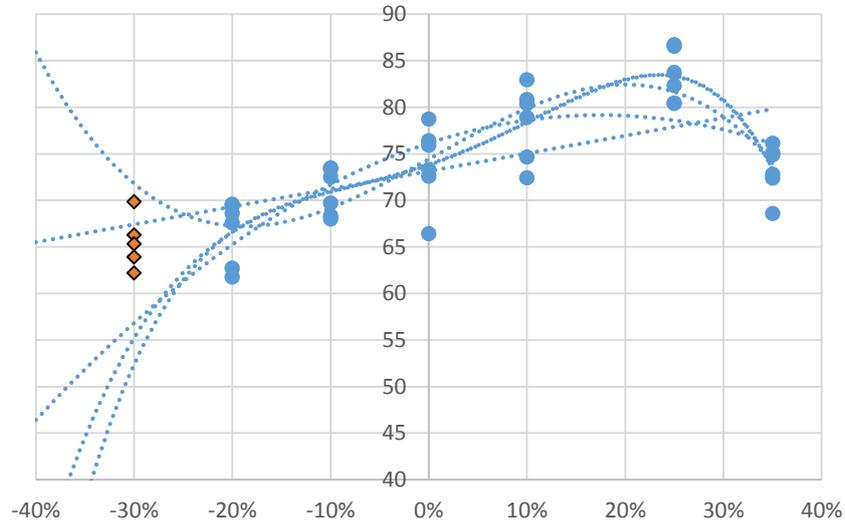
**Fig. 3. Compressive strength of bone cement with a -35 % deficiency of the liquid component: comparison of mathematical models and experimental data**
