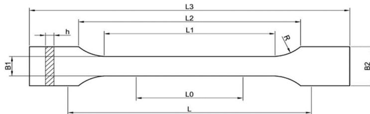
Fig. 3. Scheme of sample in accordance with PN-EN ISO 527 standard
