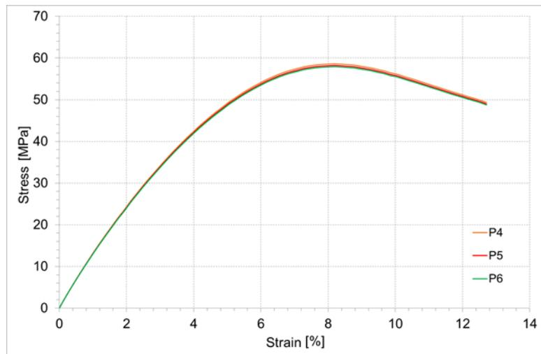
**Fig. 6. Engineering stress vs. engineering strain characteristics for tensile test of Clear resin**
