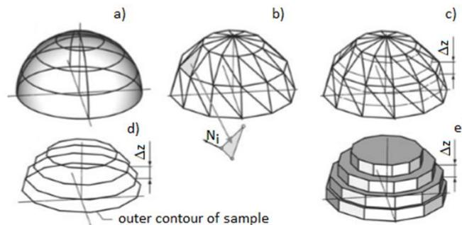
**Fig. 1. Stereolithographic model creation process: a) CAD model, b) STL model, c, d) division of STL model into layers, e) ready SLA model;  $\Delta z$  – thickness of single layer of SLA model,  $N_i$  – normal vector (Kowalska-Bany & Krokosz, 2008)**
