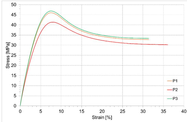
**Fig. 5. Engineering stress vs. engineering strain characteristics for tensile test of Tough resin**
