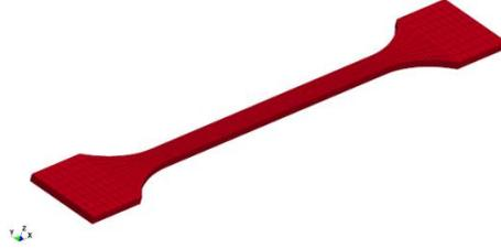
Fig. 7. Numerical model of a paddle sample
