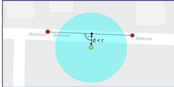
**Fig. 4. The situation, in which the points of occurrence of an object have the location data that is not within the direct range of the given street lamp – however, based on the appropriate mathematical calculations, the algorithm recognizes the presence of an object within the area of the street lamp**
