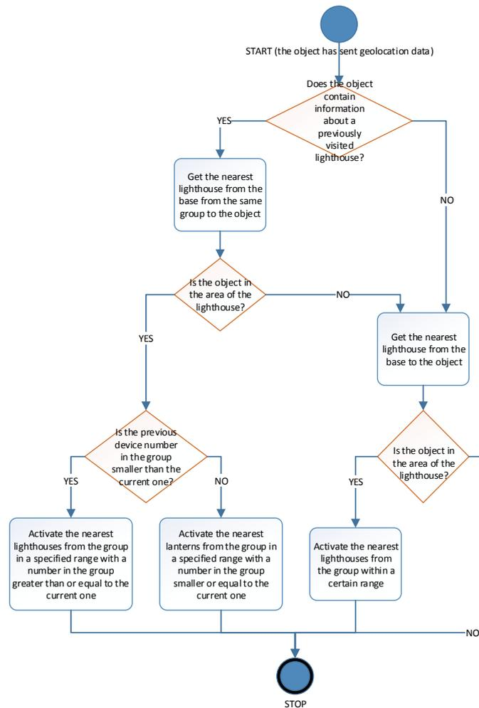
**Fig. 6. A block diagram of an algorithm that activates street lamps, after receiving data about an object moving towards this lamp – in the case of pedestrians, it is not necessary to check the state of the previous lamp number within the group of lamps**
