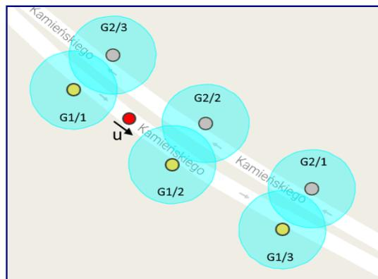
**Fig. 5. The situation, in which there are street lamps on both sides of a two-directional road – the algorithm will activate only the correct set of available street lamps on one side of the road, based on determining a given lamp group number and its sequential number within a given group**
