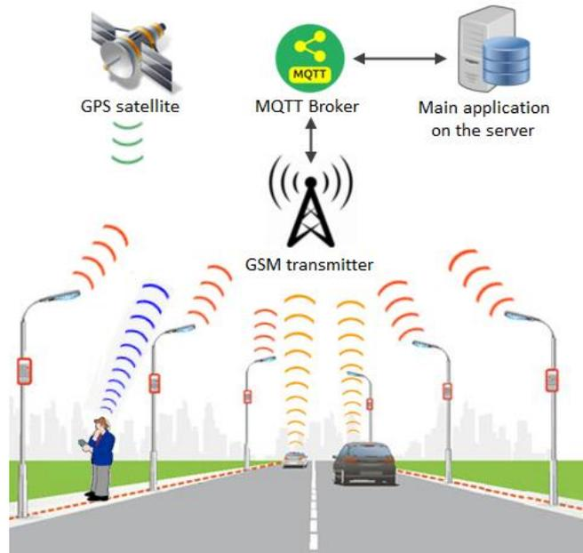
**Fig. 2. Scheme of data exchange between objects in the system and the server – in the GPS technology users' and vehicles' mobile devices transmit their current locations to the server, and this allows for the management of street lamps by a central application**
