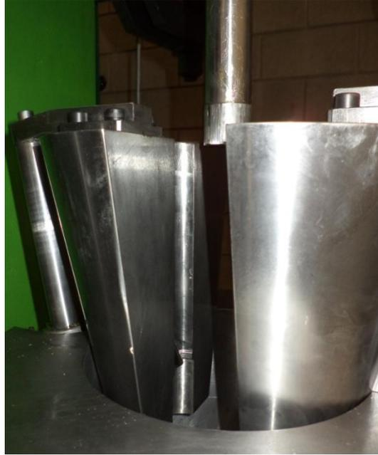
**Fig. 11. Apparatus for split-die extrusion of twist drills**
