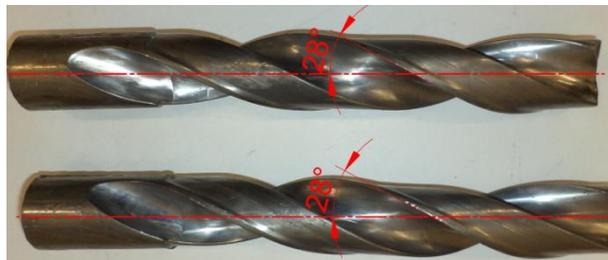
**Fig. 12. Twist drills obtained in the experiments**
