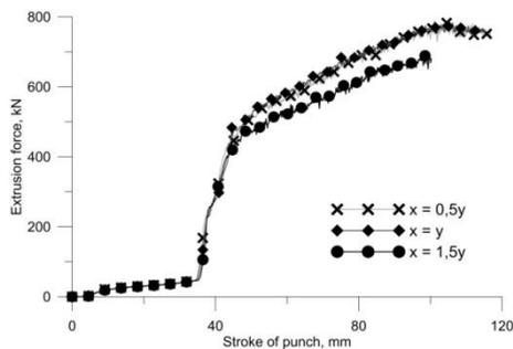
Fig. 9. A curve of punch extrusion forces
