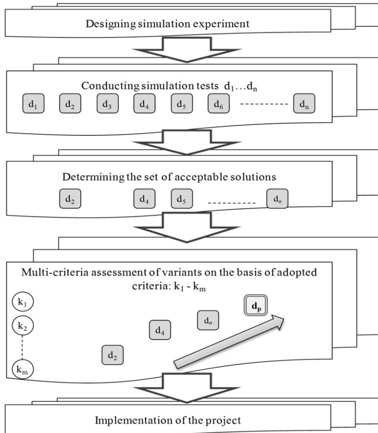
**Fig. 3. Simulation experiment and multi-criteria assessment of variants**
