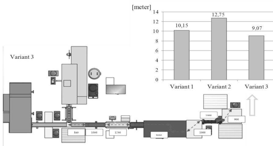
Fig. 6. Distance covered by a product on a line
