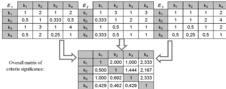
**Fig. 9. Criteria significance assessment using the Saaty's method for three experts and an overall matrix of criteria significance**
