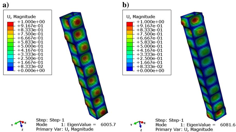
**Fig. 5. Modes of instability and critical forces (eigen value) for the following ply orientations: a) K5-90/0/45/45/0/90, b) K6-90/45/0/0/45/90 [source: own study]**
