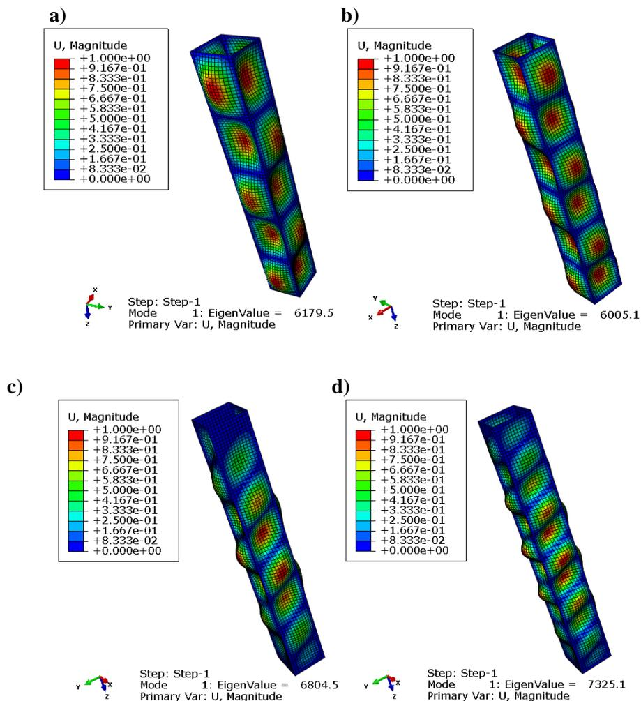
**Fig. 4. Modes of instability and critical forces (eigen value) for the following ply orientations:**
