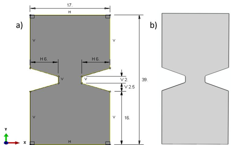
**Fig. 1. Test specimen: a) geometric dimensions, b) numerical model with internal fillets at 0.5 mm narrowing [source: own study]**
