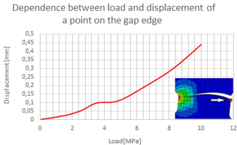
**Fig. 7. Load characteristics versus crack initiation point displacement [source: own study]**
