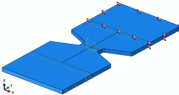
**Fig. 3. Boundary conditions of the numerical model [source: own study]**
