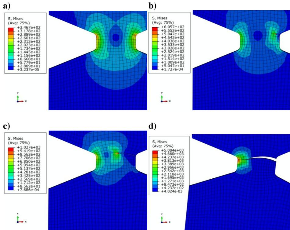
Fig. 5. Crack initiation and propagation [source: own study]
