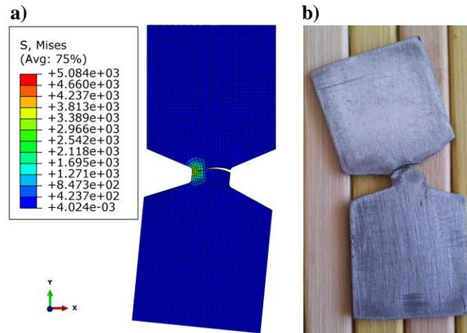
**Fig. 8. Comparison of cracking in numerical (a) and real specimens (b) [source: own study]**
