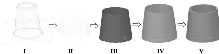
**Fig. 1. A sample procedure for geometric modelling using the scanning data [source: own study]**
