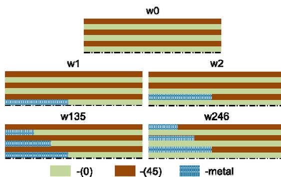
Fig. 6. Laminate configurations [source: own study]
