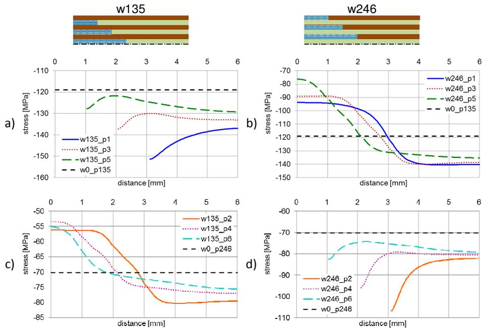
**Fig. 10. Normal stress (axial component) in laminate layers – cases w135 and w246: a)-b) layers p1,p3,p5; c)-d) layers p2,p4,p6 [source: own study]**
