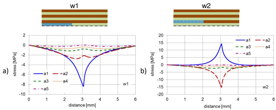
**Fig. 9. Shear stress in adhesive layers – cases w1 and w2 [source: own study]**
