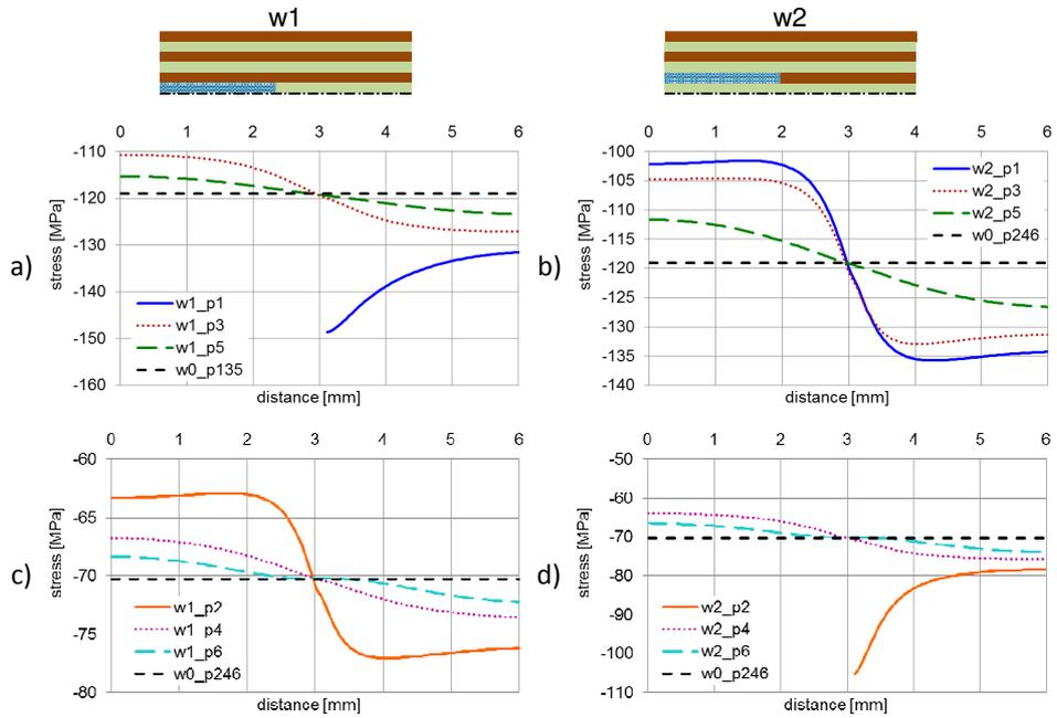
**Fig. 8. Normal stress (axial component) in laminate layers – cases w1 and w2: a)-b) layers p1,p3,p5; c)-d) layers p2,p4,p6 [source: own study]**
