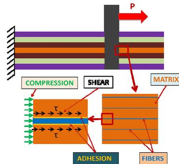
**Fig. 2. Load transfer in mechanical joint of fibre reinforced composite**
