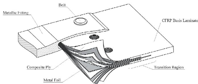
**Fig. 3. Titanium foils bonded between laminate layers [2]**
