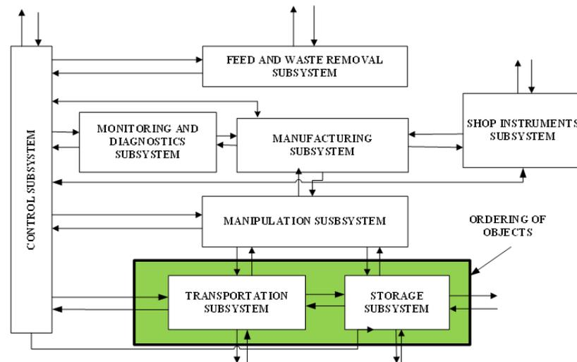
**Fig. 1. FMS structure [12]**
